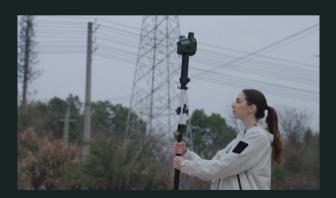
Self-developed RTK-SLAM technology: In conjunction with a telescopic pole, enables full-range high-precision RTK data collection, with accuracy <5 cm in 1 minute without GNSS.
